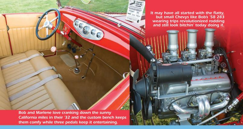
One of the coolest features of the roadster is that the interior and exterior blend together to create the overall look. The interior starts with the Auburn-style dash with a turned insert holding Stewart Warner gauges. A custom drop holds the stock column, turn signal indicators, and the system is topped with a four-spoke wheel. Costa Mesa Auto Upholstery was put in charge of fabricating the custom bench seat and covering it with tan leather in addition to laying down the short nap
